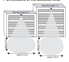
At maximum sensitivity and angle of incidence
