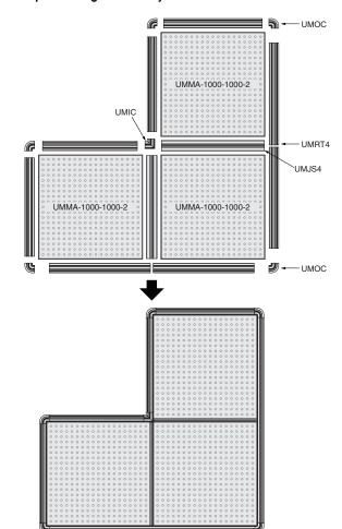
In this case, the perimeter of the Safety Mat is about 8 m, the joint between the Safety Mats is 2-m long, and the following pieces are required:
