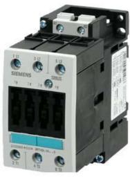
CONTACTOR, AC-3 18.5 KW/400 V, AC 230 V, 50 HZ, 3-POLE, SIZE S2, SCREW CONNECTION
