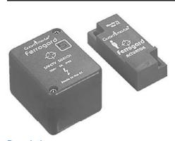
The Ferrogard range of magnetically actuated switches offers noncontact reliability together with tolerance to misalignment. They are designed to be installed so that when a guard door is opened, the action of the magnetic actuator being removed from the switches opens the N.C. safety contacts which are intended for the isolation of control power to a machine primary control element.
