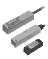
The Ferrogard range of magnetically actuated safety switches offers non-contact reliability together with tolerance to misalignment. They are designed to be installed so that when a guard door is opened, the action of the magnetic actuator being removed from the switch opens the N.C. safety contacts which are intended for the isolation of control power to a machine primary control element.
