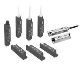
The Ferrogard range of magnetically actuated safety switches offers non-contact reliability together with tolerance to misalignment. They are designed to be installed so that when a guard door is opened, the action of the magnetic actuator being removed from the switch opens the N.C. safety contact which is intended for the isolation of control power to a machine primary control element.
