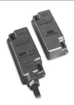
The Ferrogard range of magnetically actuated safety switches offers non-contact reliability together with tolerance to misalignment. They are designed to be installed so that when a guard door is opened, the action of the magnetic actuator being removed from the switch opens the N.C. safety contacts which are intended for the isolation of control power to a machine primary control element.
