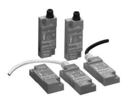
The Ferrogard range of magnetically actuated safety switches offers non-contact reliability together with tolerance to misalignment. They are designed to be installed so that when a guard door is opened, the action of the magnetic actuator being removed from the switch opens the N.C. safety contacts which are intended for the isolation of control power to a machine primary control element.
