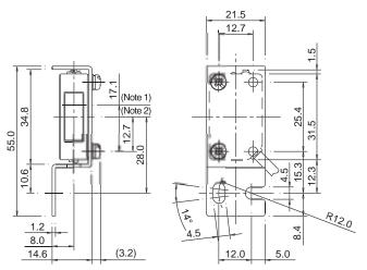
Note 1: Center of optical axis (through-beam type) Note 2: Center of optical axis (polarized retroreflective, diffuse reflective, and small-beam reflective type)
