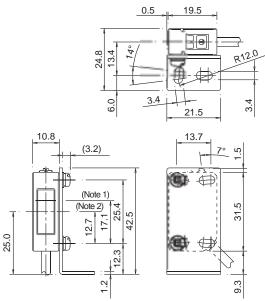
Note 1: Center of optical axis (through-beam type) Note 2: Center of optical axis (polarized retroreflective, diffuse reflective, and small-beam reflective type)
