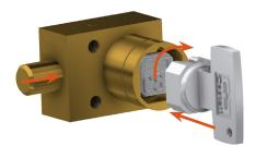
By inserting and turning the key in the bolt interlock, you can retract the bolt, e. g., releasing the disconnector. This will trap the key into the lock. 3 Key is trapped, bolt is retracted
