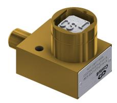
The K Lock is a key operated mechanical bolt interlock that is suitable for the control of electrical switchgear. The standard unit comes with a 15.88 mm diameter bolt available in various lengths, that is used to control the rotation or movement of operating handles or toggles of electrical switchgear. Many suppliers of switchgear equipment have mounting kits available for Castell interlocks. The lock is manufactured in brass or stainless steel.
