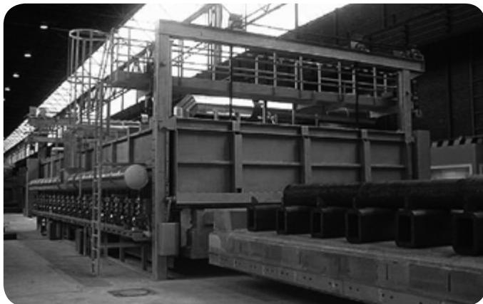
Metallurgical industry: bogie hearth furnace
