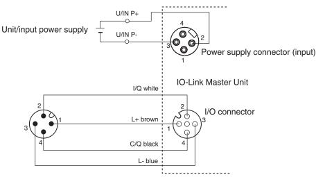
IO-Link device (with digital inputs for pin 2)
