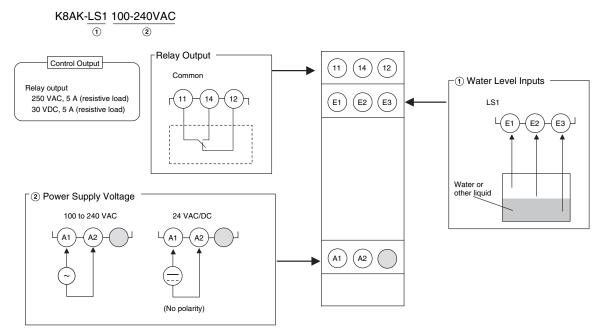
Note: 1. Do not connect anything to terminals that are shaded in gray.2. Use the recommended ferrules if you use twisted wires.
