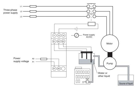
Pump motor protection mechanisms have been omitted.
