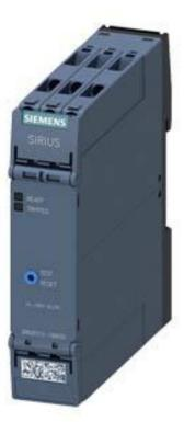
Thermistor motor protection relay Standard evaluation unit 22.5 mm enclosure screw terminal 2 change-over contacts US = 24 V-240 V AC/DC Manual/Auto/Remote reset with ATEX approval 2 LEDs (READY/TRIPPED) galvanic isolation Test/reset button Wire break monitoring Short circuit monitoring non-volatile
