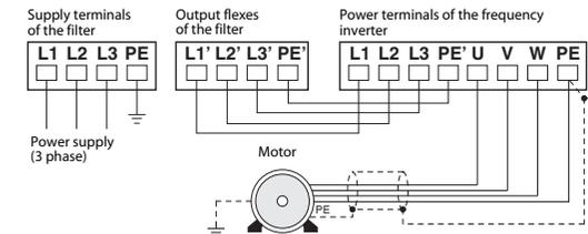
The shielded motor cable must be earthed at both ends in order to reduce radiated noise.
