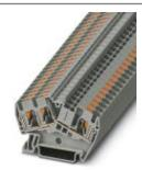
Feed-through terminal block, nom. voltage: 800 V, nominal current: 32 A, connection method: Push-in connection, number of connections: 3, cross section:0.2 mm² - 6 mm², AWG: 24 - 10, width: 6.2 mm, color: gray, mounting type: NS 35/7,5, NS 35/15
