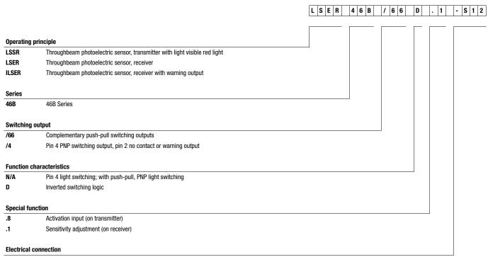
N/A Cable, standard length 2000 mm ,200-S12 Cable, length 200 mm with M12 connector
