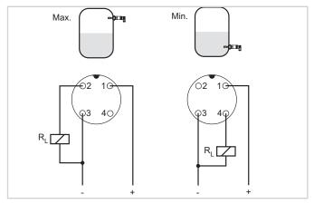
VEGASWING 51 with M12 x 1 plug connection
