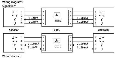
with jumper for actuators SR-,
