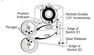
Figure 9: Switch Angle Settings
