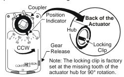
Figure 3: M91xx Actuator Components
