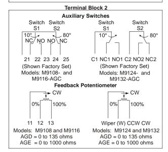
Figure 5: Wiring Diagrams for M91xx Models
