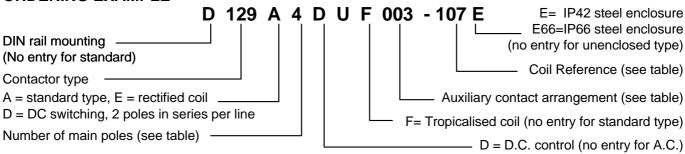
Mechanically interlocked pairs of contactors are also available. Select from the standard references below but substitute **229** for **129** in the given part number. Note that DIN rail mounting is not available on interlocked units.
