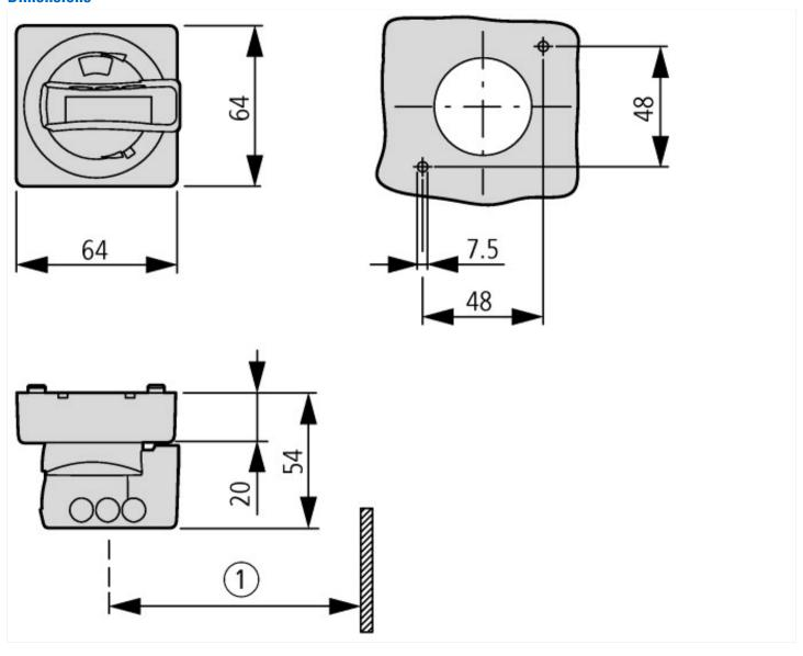
Mounting depth: 125 to 240 mm from the top edge of the top-hat rail to the front edge of the cabinet door/cover ① At least 100 mm from cover hinge
