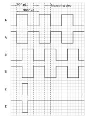
Cw with view on the encoder shaft in direction "A", compare dimensional drawing. ① Interfaces G, P, R only for channels A, B, Z.
