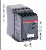
The CM-ENN UP/DOWN monitors levels of conductive liquids and media and is used e.g. for liquid level control in pump systems. The measuring principle is based on the resistance change sensed by singlepole electrodes.
