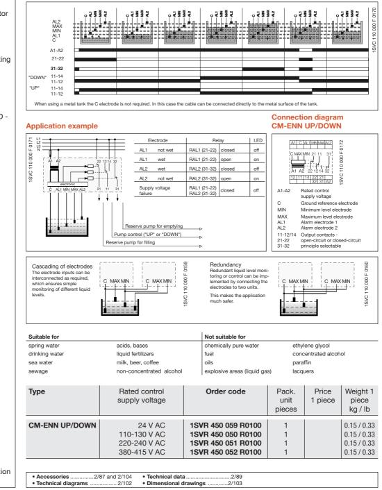
Liquid level relay with 5 electrode inputs Level control with
