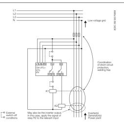
Automatized grid connection instead of a permanently accessible switching point with a disconnection function
