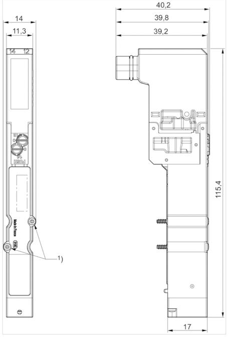
1) Mounting screw: X-slot DIN EN ISO 4757-Z0 tightening torque for mounting screw [Nm]: 0.25
