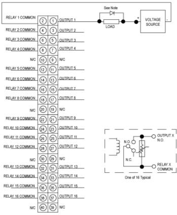
N/C Not ConnectedN.O. Normally OpenN.C. Normally Closed
