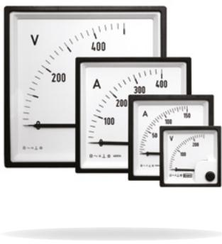
Designed to measure AC current or voltage, these meters indicate true RMS values and are substantially independent of system waveform. Scales are calibrated down to 20%, and ammeters can have overload scales of x2, x3, x5 or x6 for motor start duty. Ammeters can be supplied for use with -1 A or -5 A current transformers, whilst voltmeters can be scaled for use with voltage transformers. Meters can be used to measure DC at reduced accuracy.
