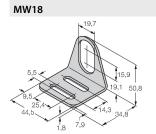
6945004 Mounting bracket for threaded barrel sensors; material: Stainless steel A2 1.4301 (AISI 304)
