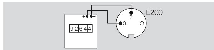
Electronic meter for digital remote indication of the current flow rate (in m<sup>3</sup>/h).
