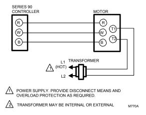
Fig. 5. Typical Series 90 Wiring.
