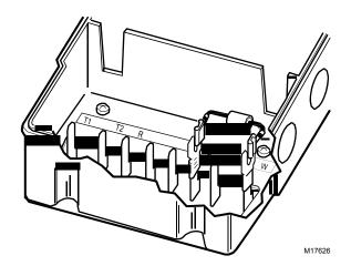
Fig. 12. Attaching a Shunt Resistor to TRADELINE Motors.
