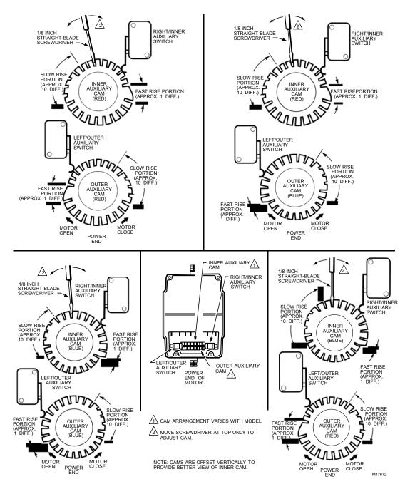
Fig. 13. Auxiliary Switch Adjustment.
