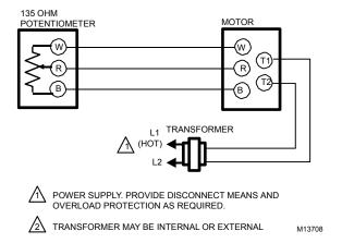
Fig. 6. Wiring for Potentiometer Control
