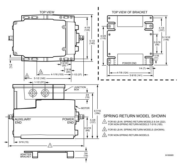
Fig. 2. Modutrol IV Motor mounting dimensions in inches (mm).
