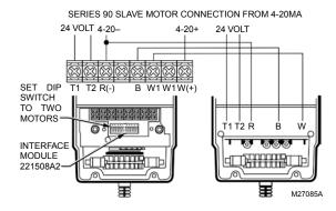
Fig. 8. Series 90 Slave Motor Connection.
