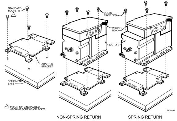
NOTE: When no bracket is used in replacement applications, damper linkages require adjustment for the new shaft position.
