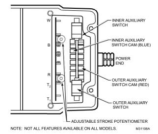
Fig. 11. Terminals and Adjustments.
