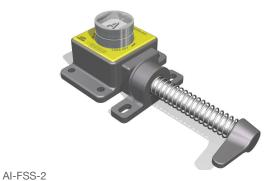
The AI is a single key access interlock ideal for use on hinged doors. The interlock has an open cavity design manufactured in either aluminium alloy/brass or stainless steel, making it ideal for use in harsh or corrosive environments and heavy use. Typical industries using the AI are food, chemical, pharmaceutical, mining, steel and power generation.
