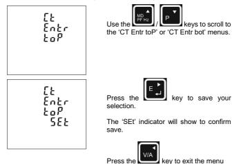
Select either BOT or TOP on each meter according to the orientation of the line phases - See diagram for example Selections BOT or TOP will automatically switch L1 to L3 (TOP) or L3 to L1 (BOT) in line with RJ CT label shown below.
