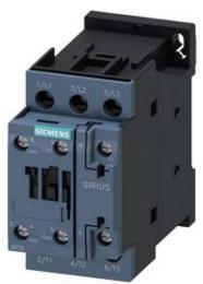
CONTACTOR, AC-3, 18.5KW/400V, 1NO+1NC, AC 230V 50HZ, 3-POLE, SZ S0 SCREW TERMINAL
