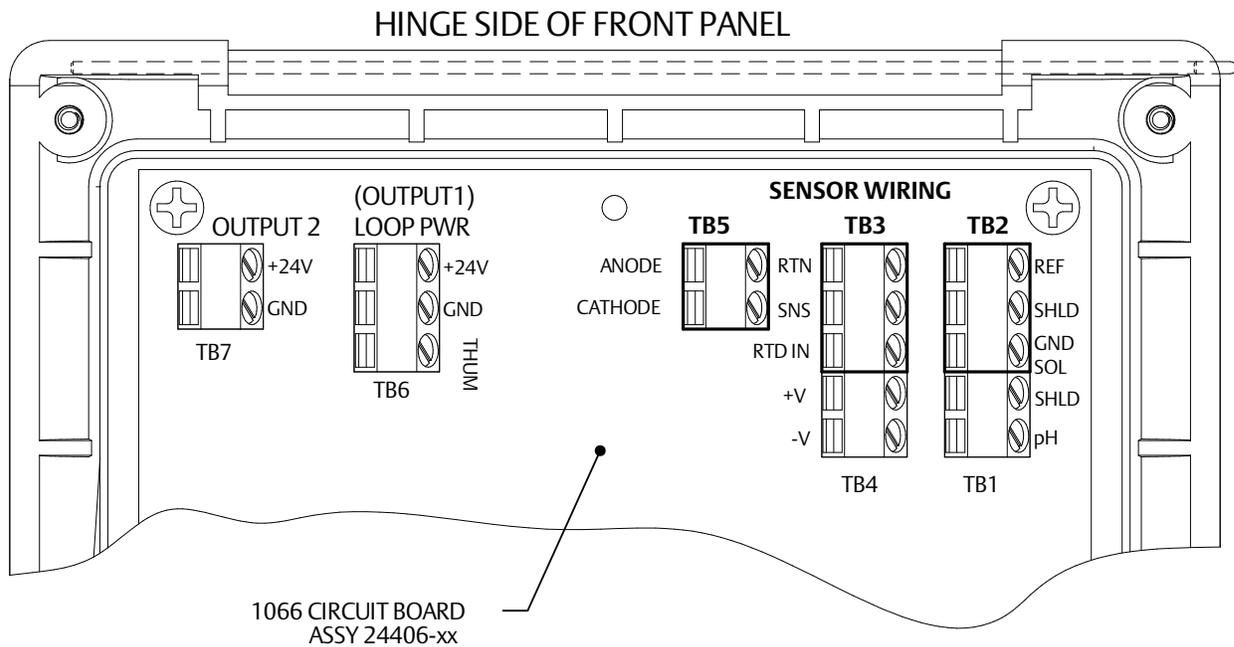
**CHLORINE, OXYGEN, OZONE SENSOR WIRING**
