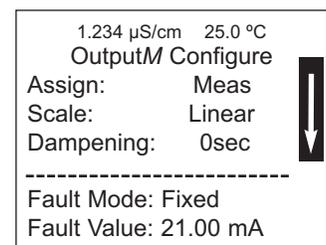
FIGURE 7-1. Configuring and Ranging the Current Outputs
