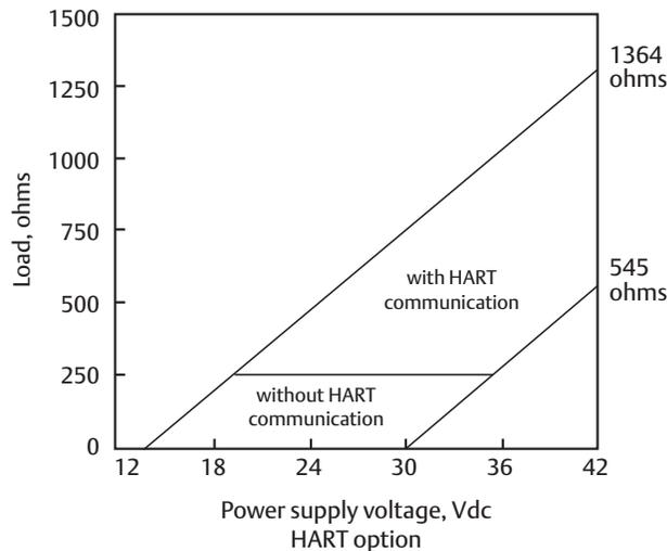
Analog Outputs: Two-wire loop powered (Output 1 only). Two 4-20 mA electrically isolated current outputs (Output 2 must be externally powered). Superimposed HART digital signal on Output 1. Fully scalable over the operating range of the sensor.
