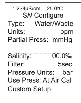
The following sub-sections show the initial display screen that appears for each configuration function. Use the flow diagram for oxygen programming at the end of Sec. 6 and the 1066 live screen prompts for each function to complete configuration and programming.
