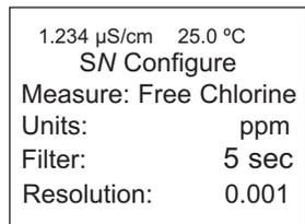
The following screen format will appear (factory defaults are shown). To program any displayed function, scroll to the desired item and press ENTER.
