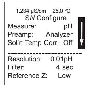
The following sub-sections provide you with the initial display screen that appears for each configuration function. Use the flow diagram for pH programming and the 1066 live screen prompts for each function to complete configuration and programming.
