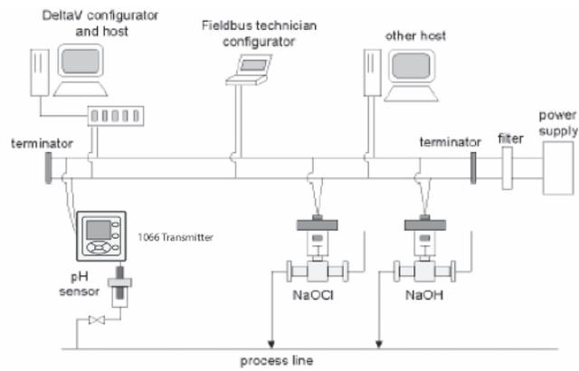
FIGURE 4-5. Typical Fieldbus Network Electrical Wiring Configuration
