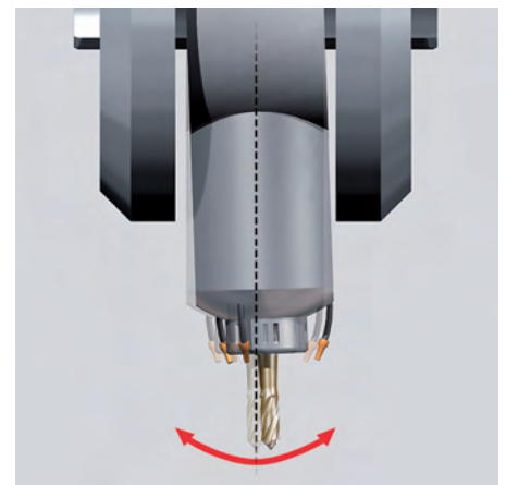
Fault characteristics according to ISO 230-1: EBA
