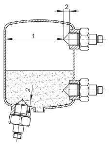
The apex should protrude into the container ① Distance  $\ge 40 \text{ mm}$
