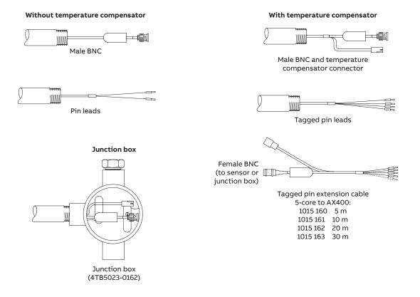
Sensor cables and junction box wiring
