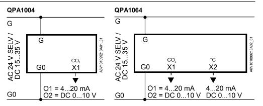
G System potential AC 24 V (SELV) or DC 15...35 V G0 System neutral and measuring neutral X1, X2 Signal output DC 0...10 V or 4...20 mA
