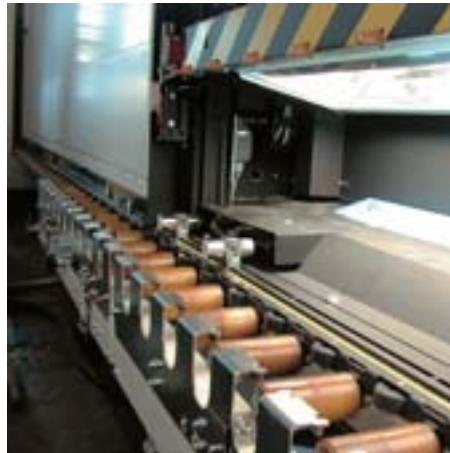
Top: insulating glass-production line fitted with Bernstein capacitive sensors
