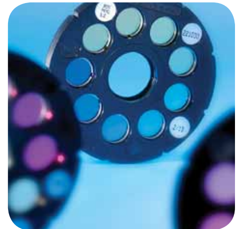
Test disc with colour-stable glass standards
