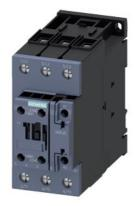
power contactor, AC-3e/AC-3, 65 A, 30 kW / 400 V, 3-pole, 175-280 V AC/DC, 50/60 Hz, with integrated varistor, auxiliary contacts: 1 NO + 1 NC, screw terminal
