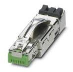
RJ45 connector, degree of protection: IP20, number of positions: 8, 1 Gbps, CAT5 (IEC 11801:2002), material: Zinc die-cast, connection method: IDC fast connection, connection cross section: AWG 26- 24, cable outlet: straight
