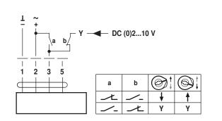
Override control (frost protection circuit)
