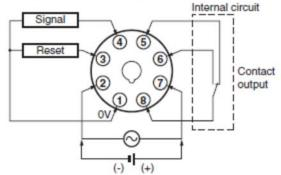
Recommended socket Model P3G-08 (sola separately) is needed.
