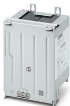
Energy storage device, LI-ION technology, 24 V DC, 120 Wh, for ambient temperatures of -20°C ... 60°C, automatic detection and communication with QUINT UPS-IQ
