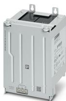
Energy storage device, lead AGM, VRLA technology, 24 V DC, 7.2 Ah, tool-free battery replacement, automatic detection, and communication with QUINT UPS-IQ
