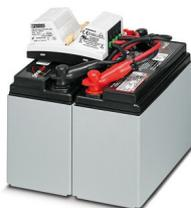
Energy storage device, lead AGM, VRLA technology, 24 V DC, 13 Ah, tool-free battery replacement, automatic detection, and communication with QUINT UPS-IQ
