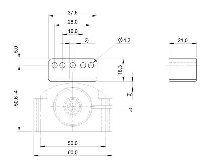
1) not included in scope of delivery, 2) Lateral offset, 3) Distance to BTL
