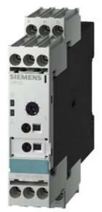
Timing relay, Multifunction Phased-out product !!! For further information, please contact our sales department 1 change-over contact, 8 functions 15 time ranges (0.05 s-100 h) 24...240 V AC/DC at 50/60 Hz AC with LED, Screw terminal
