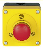
E-STOP/contact block incl. Surface mount housing, set consisting of E-STOP pushbutton with E-STOP symbol and with logo and contact block with monitoring, 2 N/C, terminals of screw type.
