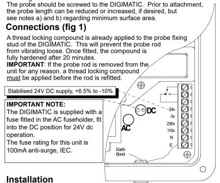
DIGIMATIC will operate on 110V/230V ac 50/60Hz or 24V dc supplies. The unit may be wired in ordinary un-screened cable of any length and need not be separated from other cables.
