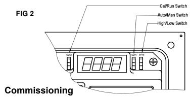
The DIGIMATIC can be calibrated automatically, manually or by a combination of the two methods. Usually, automatic calibration is the simplest method, particularly when the vessel can be filled to cover the probe. Manual calibration is useful when a number of probes in similar applications need to be set. Once the correct calibration has been determined and noted, on one system, the remainder can be set to the same setting.
