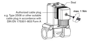
Cable plug can be rotated 4 x 90°.
