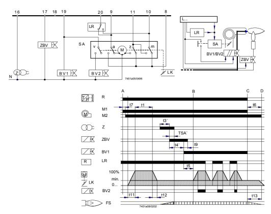
The air damper is kept closed during burner off periods. For other connections, refer to «Connection diagrams».
