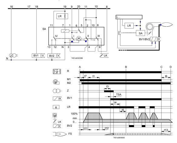
Control of actuator «SA» according to the single-wire principle (actuator «SA»: E.g. SQN3... as per Data Sheet 7808). For other connections, refer to «Connection diagrams».
