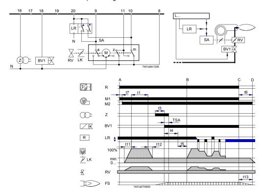
The air damper is kept closed during burner off periods. For other connections, refer to «Connection diagrams».
