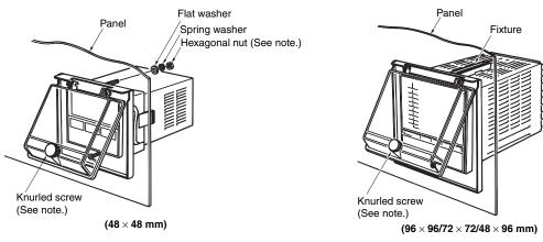
Note: Tighten the knurled screw to a torque of 0.02  $N \cdot m$  and the hexagonal nut to a torque of 0.05  $N \cdot m$ .
