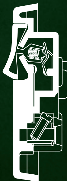
Unique labyrinth switch design minimises visible arc flash and prevents front access to live parts.
