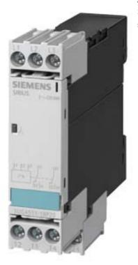
Analog monitoring relay Phase sequence monitoring 3 x 320...500 V 50...60 Hz AC 2 change-over contacts screw terminal Successor product for 3UG3511-1BQ50
